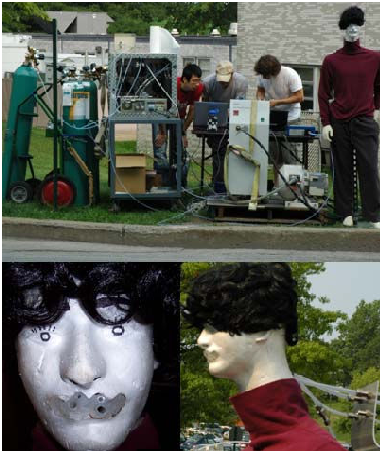
Figure 1 Mannequin and test setup. The top photograph shows the emissions measurement equipment and the mannequin alongside the test road. The bottom photographs show the mannequin's head with sample tubes in the mouth and their attachment to the transport tubing.
